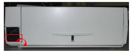
5. Align and insert new fuses in plastic fuse tray.
